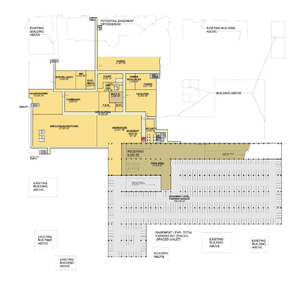
BASEMENT LEVEL FLOOR PLAN
